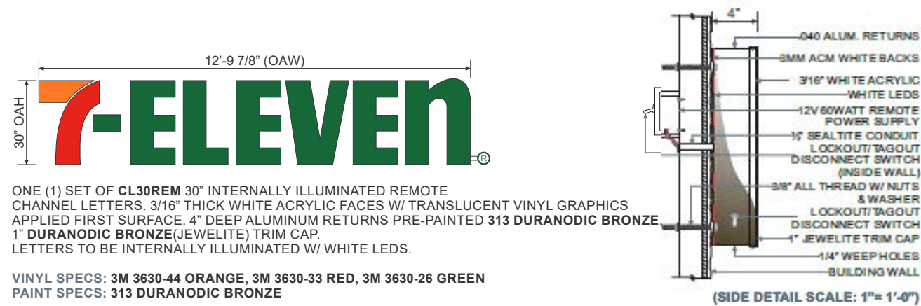
Front View & Side Mounting Detail - CL30REM 30" Internally Illuminated Remote Channel Letters - Sign A 1/4" = 1'-0" Display Square Footage: 32.0
